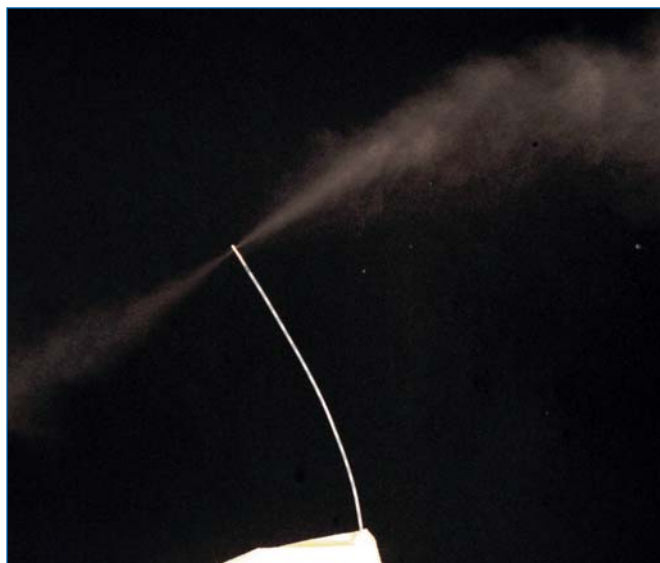
Figure 4. Steam is ejected from two areas at the tip of the catheter.
